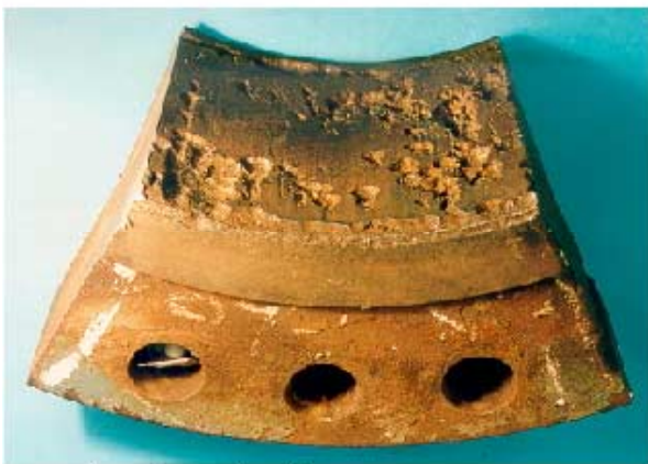
Corrosion of vessel wall
