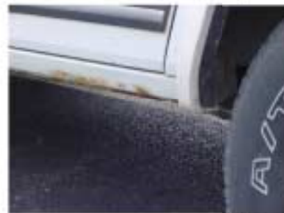
Corrosion under damaged coating
