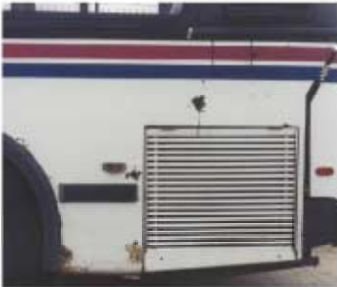
Area of corrosion on a bus
