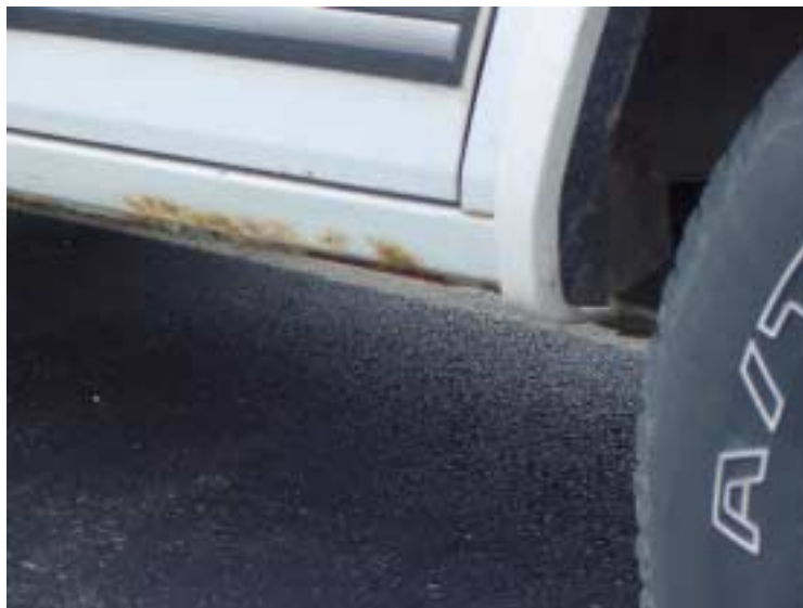
Figure 1. Example of general corrosion of painted steel automobile body panel.
