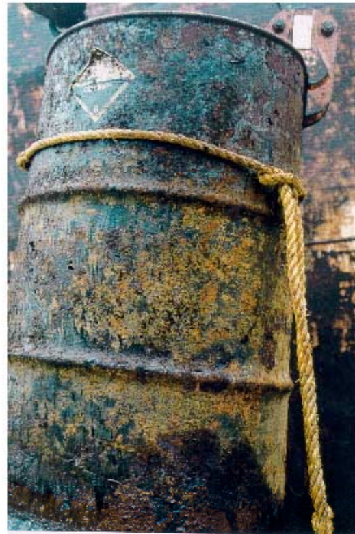
Corroded storage drum
