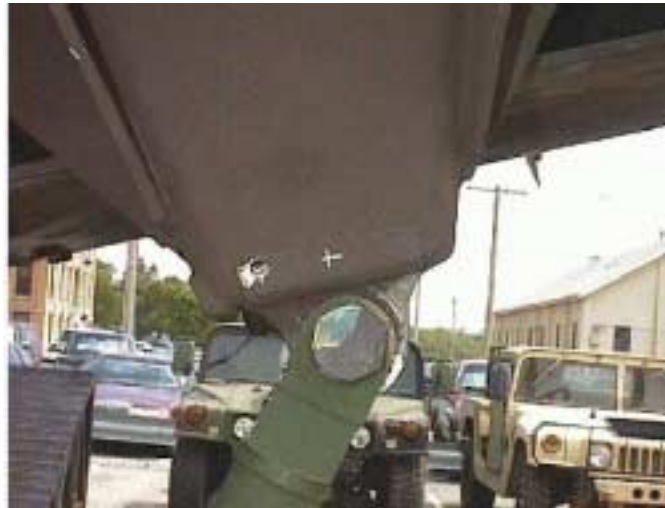
Figure 4. Drainhole in M198 towed howitzer.
