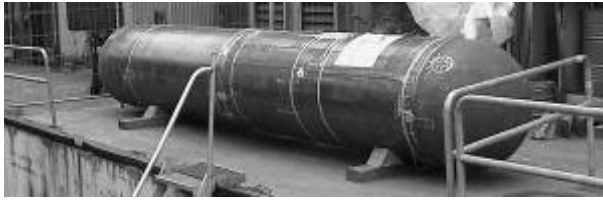
Figure 15: Full scale end-capped test pipe at Europipe's test site
