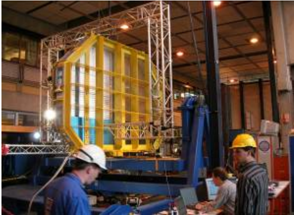
Figure 4: Test rig with 1:10 scale model for the ComFLOW 2-phase JIP
